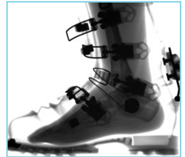
Biplanar X-ray images are collected to assess the effect of canting insoles on skeletal alignment inside the ski boot
