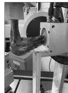
Fig 1. Biomechanical setup with the humerus secured to a custom-designed fixture
